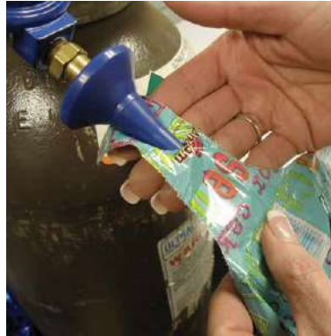
Insert the foil nozzle carefully into the valve opening.
