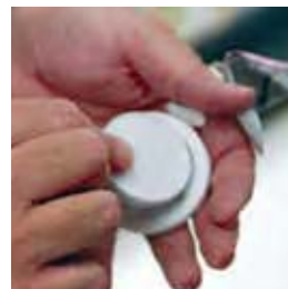
Match the notches on the spool to the grooves on the adapter
